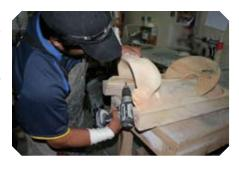
In addition to parts that are PRECISION cut on our CNC machine, our trees are now constructed in a *new*, Unique Combo-Jigging System. Our new Jigging System ensures the swells and cantle are properly centered on the bars and the horn is centered on the swell. We don't eye ball 'em!
