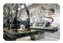
We use three-dimensional scanners and computer aided design (CAD) software to engineer parts which are cut on CNC machines. This equipment allows us to produce parts that are the same each and every time.
